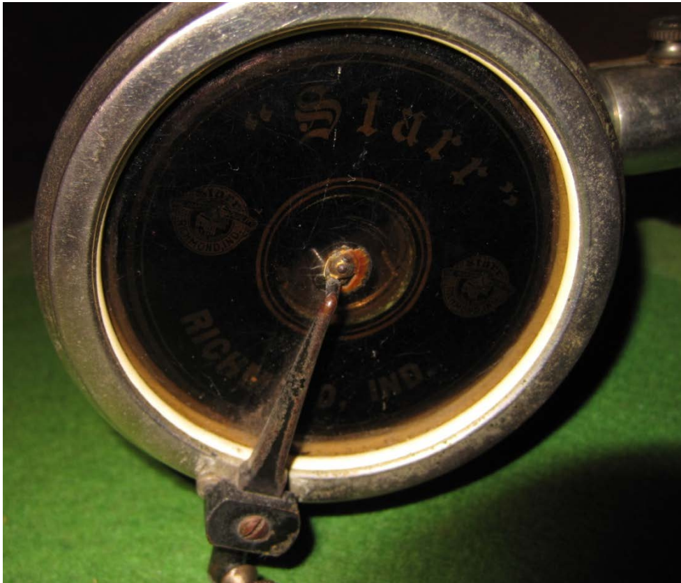
Early Starr Sound Box -- Stylus Bar is Pivot Mounted
