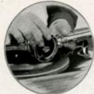
Fig. 2 shows Reproducer immediately after locking pin has been put in groove, from which position it can be turned to the left for the three different playing positions.
